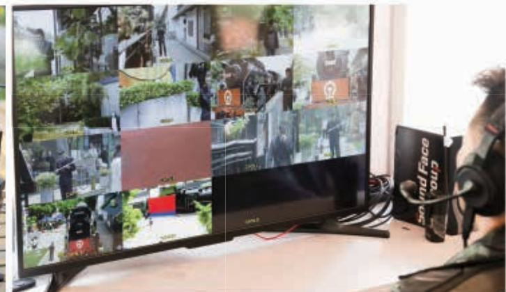
14x FLOW wireless Rx for director monitoring, without interference to each other.
