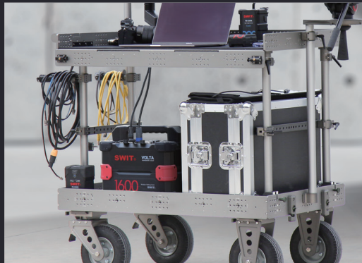
Film Cart Power Center Monitors, cameras, wireless Rx, Laptops
