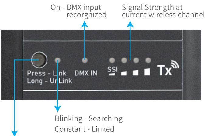
Press the link button on the Tx, to link all Rx in the receiving environment.
