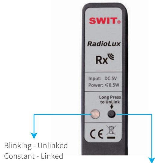
long press the unlink button will unlink this single Rx from the Tx in the system.
