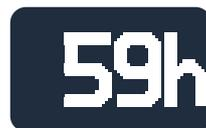
If the working time is less than ten hours, it will display 0~9:59; If the working time is more than 10 hours, it will display remaining working hours.
